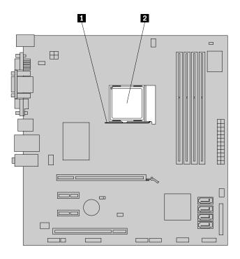
Figure 33. Accessing the microprocessor
